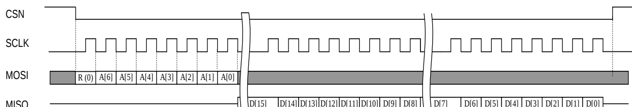
Figure 14: SPI read procedure
