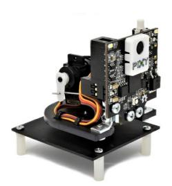
Bazaar / Robotics & CNC / Other for Robotics & CNC / Pan/Tilt2 Servo Motor Kit for Pixy2 - Dual Axis Robotic Camera Mount
