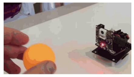
This is a kit for a pan/tilt mechanism designed specifically for Pixy2. Assemble the kit, connect Pixy2 (sold separately), and start following colored objects using the Pan/Tilt demo in F download). It includes two durable laser-cut plastic pieces for the base, two servos for the pan and tilt axes, and all the mounting hardware and cable ties you need to assemble. As are located on our wiki.
