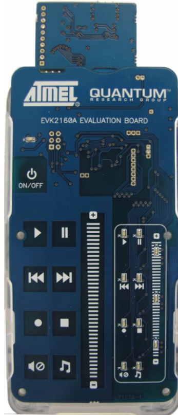
Figure 1-6. USB Plug-in Card and EVK2160A Setup Complete
