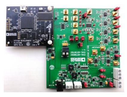
The **EVAL-AD7367SDZ** evaluation board is a member of a growing number of boards available for the **SDP**. It was designed to help customers evaluate performance or quickly prototype new **AD7367** circuits and reduce design time.
