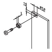
Sleeve guides the collar screw when fastening the front panel.
