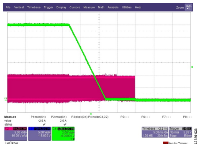
Figure 36. Soft Stop with SR on Time Extension (8 ms) Green Trace: Output Voltage Red Trace: SR1
