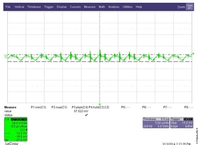
Figure 53. Output Voltage Ripple, 20 A Load Green Trace: AC Coupled Output Voltage
