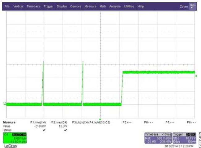
Figure 39. Recovery from VOUT_OV_FAST_FAULT Green Trace: Output Voltage
