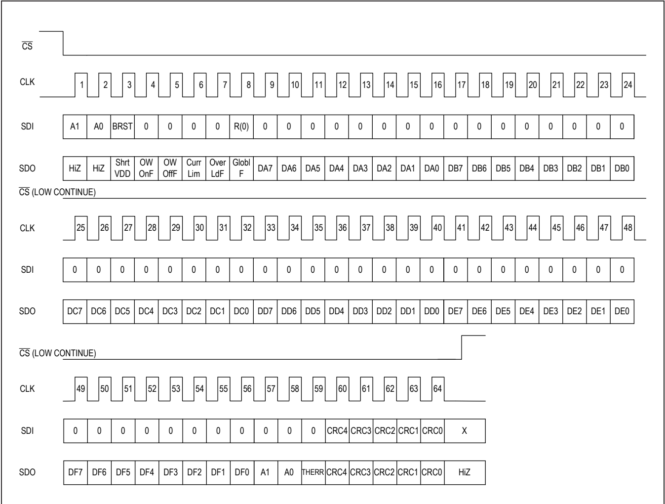
Figure 16. Addressed SPI Burst Read Command with CRC
