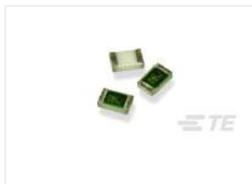
TE Part #5-1676481-9 CPF 0603 1K6 0.1% 25PPM 1K RL
