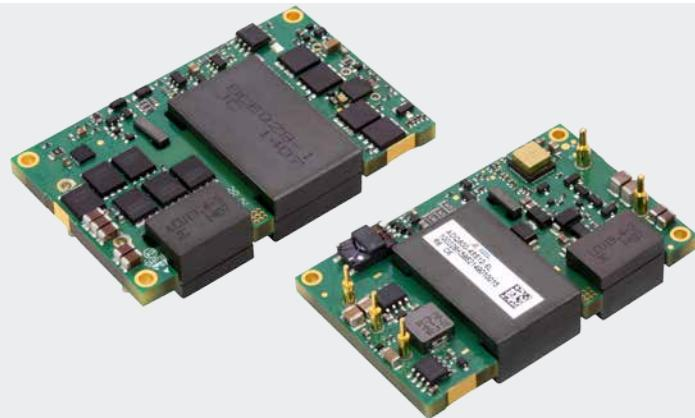
Advanced Energy's Artesyn ADQ600 series quarter-brick isolated DC-DC converter produces a single fully regulated 12 V output. Rated at 600 watts, the converter can deliver up to 50 amps output current and has no minimum load requirement. It has an input voltage range of 40 to 60 V and is primarily designed for use with standard 48 V supplies in computing and server applications, as well as regulated 48V supplies in telecommunications equipment.
