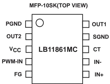
VCC: Common power supply for motor and control systems
