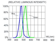
FIG.4 RELATIVE LUMINOUS INTENSITY VS. WAVELENGTH.
