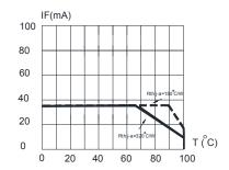
FIG.5 Blue MAXIMUM FORWARD DC CURRENT VS AMBIENT TEMPERATURE (Tjmax=110℃)
