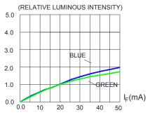
FIG.2 RELATIVE LUMINOUS INTENSITY VS. FORWARD CURRENT
