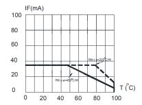
FIG.5 Green MAXIMUM FORWARD DC CURRENT VS AMBIENT TEMPERATURE (Tjmax=110 $^{\circ}\text{C})$
