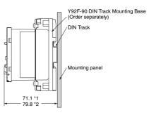
Using a PFP-50N or PFP-100N Mounting Track.
