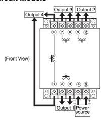
Note: 1. The Time Switch output uses a no-voltage contact. An external power supply is required for applications in which a load is driven.
