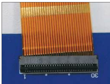
✗ Skewed FPC Insertion
