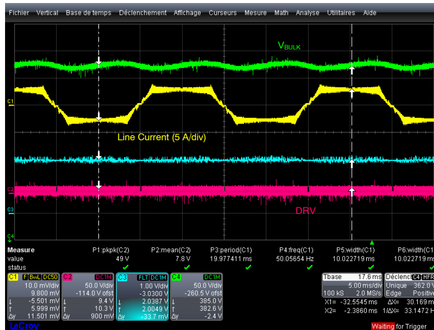
Figure 14. Over-Current Situation (85 V, 0.5 A Load Current)
