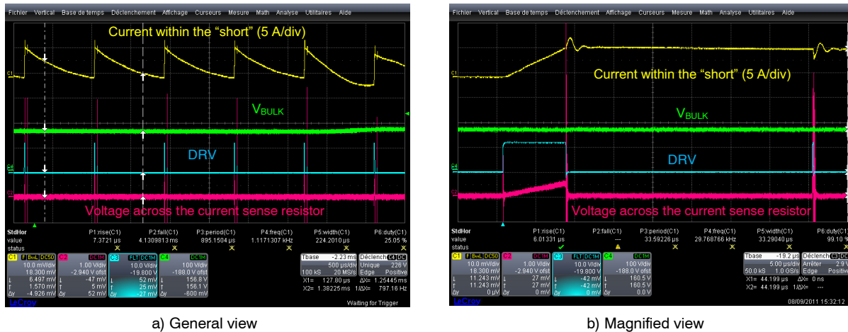
Figure 17. Shorting the Bypass Diode and the NTC
