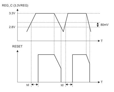
\*1 : td is the delay time. It is set by an external capacitor connected between the CD pin and ground). \*2 : The voltage at which RESET changes state is a typical value (voltage).
