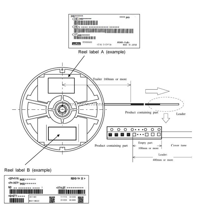
3-7-4 Other notes Continuously missing device shall not exceed 2 pcs. Peeling strength of the cover tape: 0.1 to 0.7N.
