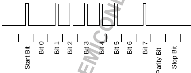
Figure 14-3. IrDA ASCII “A” Character with Odd Parity
