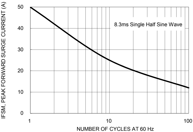
FIG. 2 MAXIMUM NON-REPETITIVE FORWARD SURGE CURRENT UNIDIRECTIONAL ONLY
