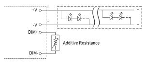
"DO NOT connect "DIM- to -V"
