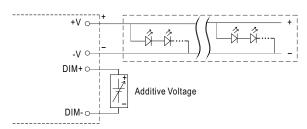
"DO NOT connect "DIM- to -V"
