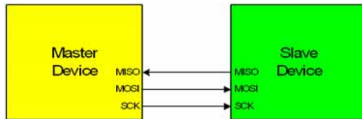
Figure 30.3. 3-Wire Single Master and 3-Wire Single Slave Mode Connection Diagram
