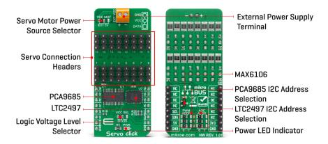
The servo can be connected to any of the sixteen headers located on this Click board™. The output signal frequency is determined by the Prescaler value, which is written to the appropriate register. The output channels can be set either in the open-drain or in the push-pull configuration. In the first case, they will be able to sink up to 25mA from up to 5V power supply, while in the second case, they will be able to both drive with up to 10mA or sink up to 25mA.
