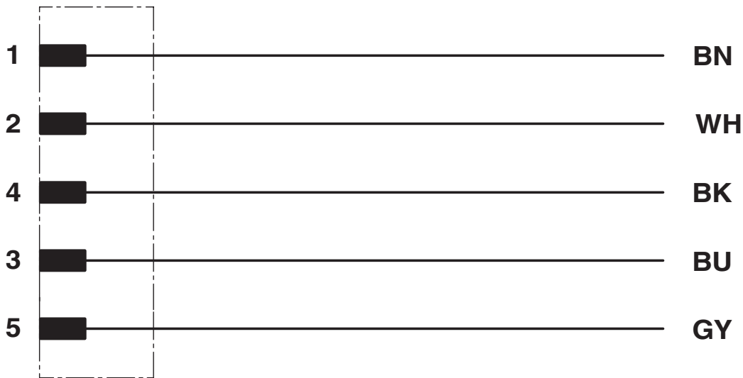
Contact assignment of the M12 plug
