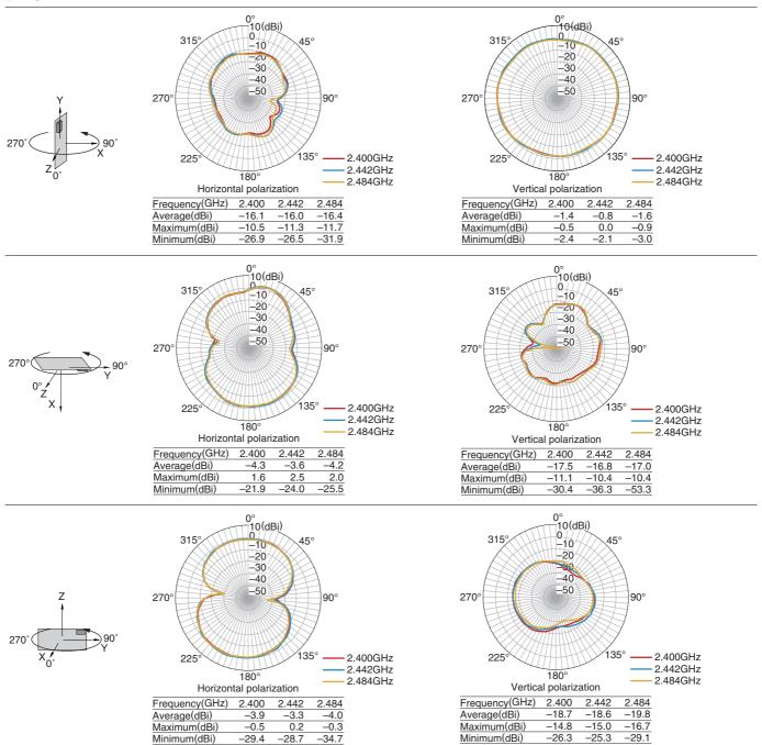
• Tested antenna has been soldered. Evaluation board size is 50x10x1 mm.
