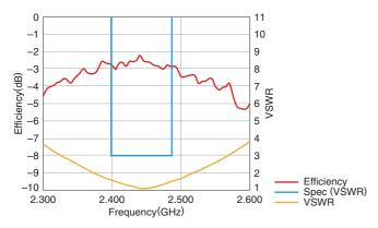
• Tested antenna has been soldered. Evaluation board size is 50x10x1 mm.
