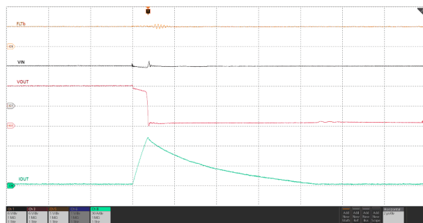
Figure 7-43. Circuit-Breaker Response TPS25974x
