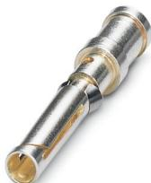
Crimp contact, contact diameter: 1.6 mm, turned, Socket, contact material: Copper alloy, contact surface: silver-plated, connection cross section: 2.5 mm<sup>2</sup> ... 2.5 mm<sup>2</sup>, AWG 14
