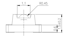
For reflow soldering (propose)
