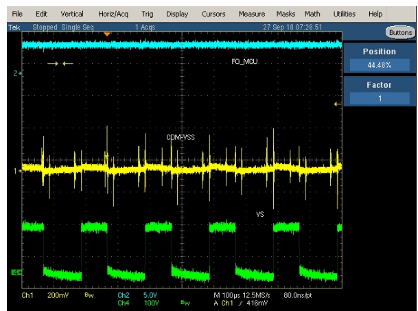
Figure 35. During startup current is high, with cap between COM-V SS , noise is less, fault conditions do not occur, compressor will not stall, 100μs/div
