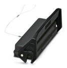
Protective cover B24, with single locking latch, protective cover material: PA, height: 21.6 mm, seal: yes, diameter of retaining cord eyelet: 30 mm
