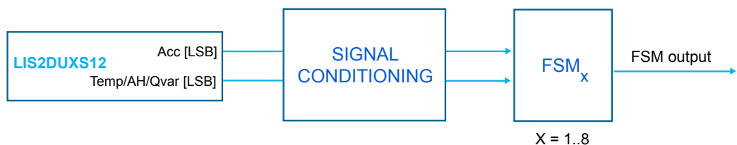
Figure 12. State machine in the LIS2DUXS12
