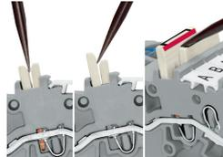
**Removing a staggered jumper:**
