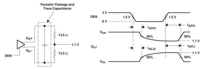
Figure 10. Serializer High-Impedance State Test Circuit and Timing
