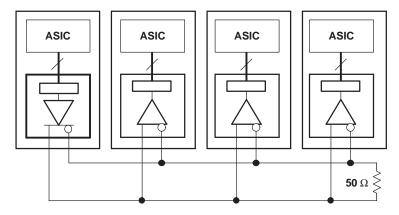
Figure 23. Multidrop Configuration
