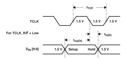
Figure 9. Serializer Setup/Hold Times
