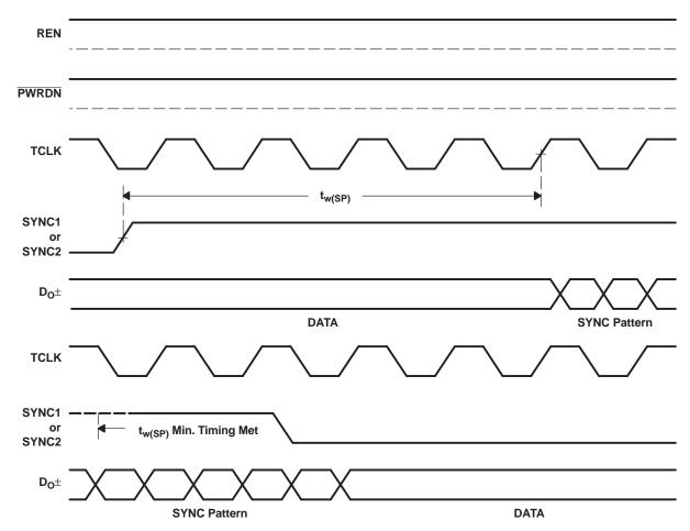
Figure 12. SYNC Timing Delays
