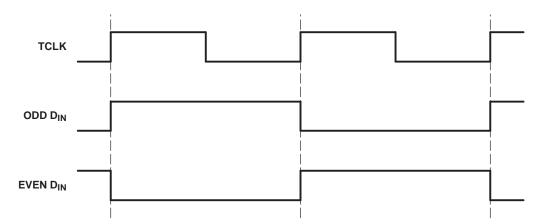
Figure 3. Worst-Case Serializer  $I_{\text{CC}}$  Test Pattern
