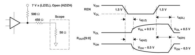
Figure 16. Deserializer High-Impedance State Test Circuit and Timing
