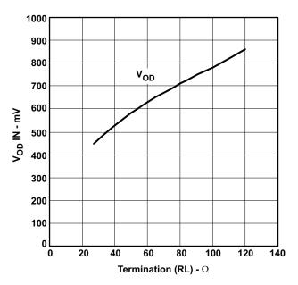
Figure 2. Typical  $V_{\text{OD}}$  Curve
