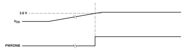
Figure 21. Device Startup
