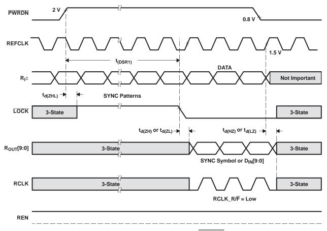
Figure 17. Deserializer PLL Lock Times and PWRDN 3-State Delays
