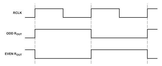
Figure 5. Worst-Case Deserializer  $I_{CC}$  Test Pattern
