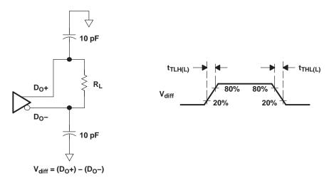
Figure 6. Serializer LVDS Output Load and Transition Times
