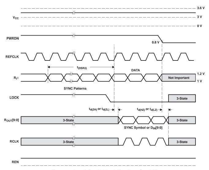
Figure 18. Deserializer PLL Lock Time From SyncPAT
