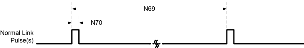
Figure 30-38. 10Base-TX Normal Link Pulse Timing
