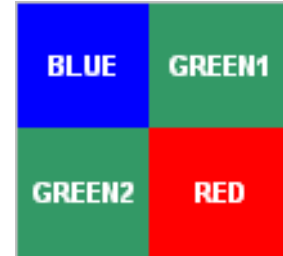
Figure 6. Color Filter Arrangement on the Pixels
