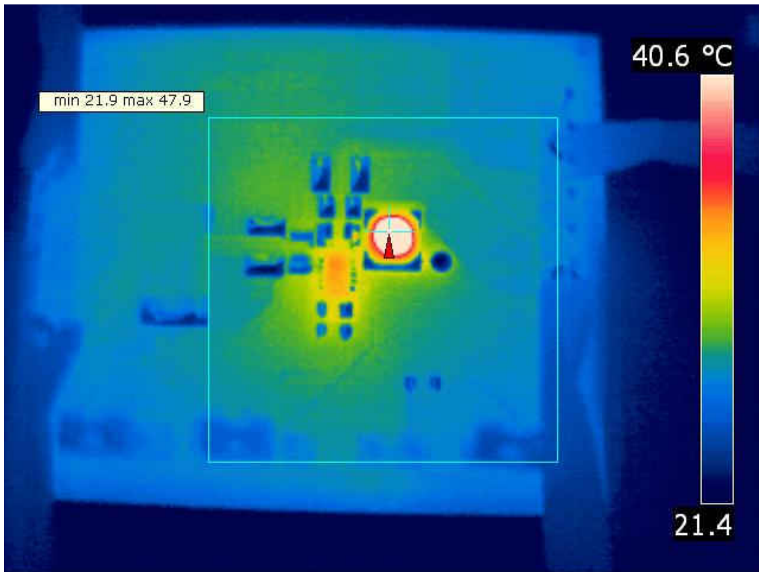
Figure 3-1. Thermal Performance ( V_{IN} = 12\text{ V} , Load = 500 mA)
