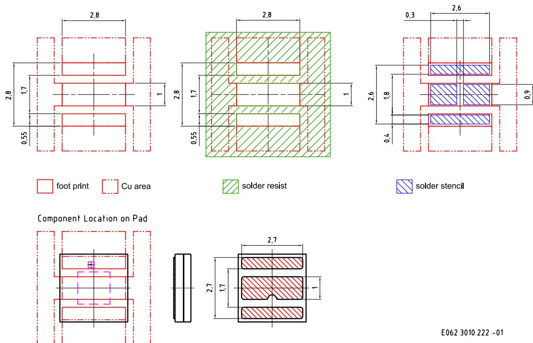
For superior solder joint connectivity results we recommend soldering under standard nitrogen atmosphere. Package not suitable for ultra sonic cleaning. To ensure a high solder joint reliability and to minimize the risk of solder joint cracks, the customer is responsible to evaluate the combination of PCB board and solder paste material for his application.
