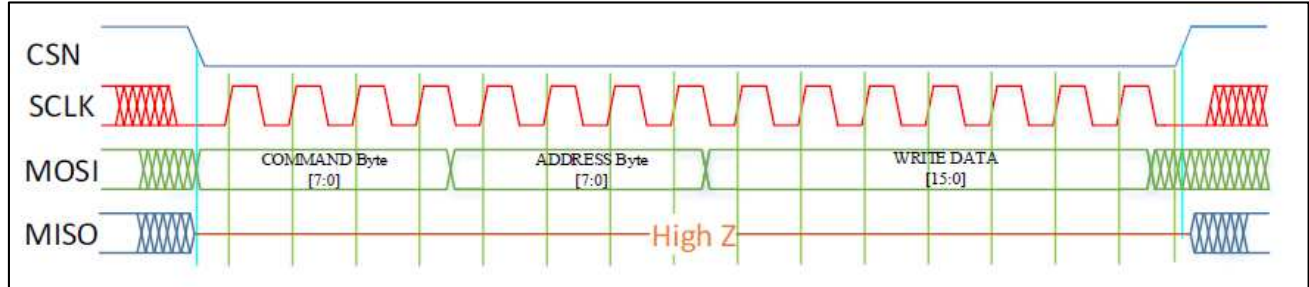
Figure 27: SPI write transfer overview
