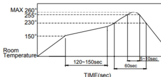
■ The condition mentioned above is the temperature on the Cu foil of the PCB surface. There are cases where board's temperature greatly differs from switch's surface be used not to allow switch's surface temperature to exceed 260°C.
