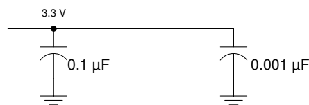
Figure 9-2. Recommended LVDS Bypass Capacitor Layout
