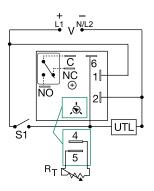
V = Voltage S1 = Initiate Switch C = Common, **Transfer Contact** UTL = Untimed Load (optional)
