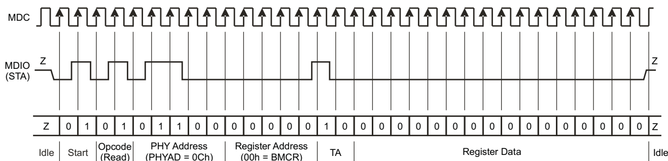
Figure 4-3. Typical MDC/MDIO Write Operation
