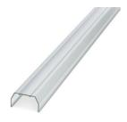
Cover profile, for covering terminal strips, snaps onto cover profile carrier AP 3-TU, AP 3-TNS 35, can be marked with insert strip AP-ES. Cover profile carriers should be placed at the ends and at intervals of approx. 40 cm. Length: 1 m
