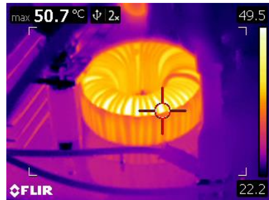
Figure 23. Thermal Scan of Inductor (1200V)
