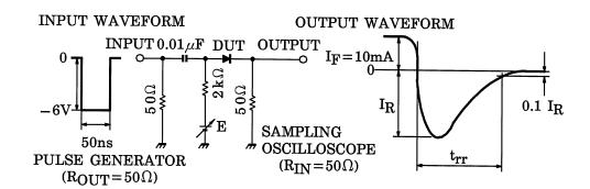
Fig.1 Reverse Recovery Time (t<sub>rr</sub>) Test Circuit
