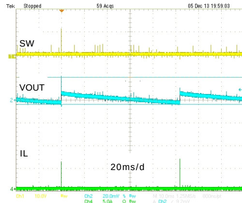
Fig. 7: V_{OUT} ripple is 22mV at 0A, DCM, 12VIN, 1.2VOUT
