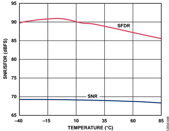
Figure 48. SNR/SFDR vs. Temperature,  $f_{IN} = 170.3$  MHz
