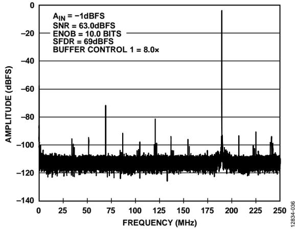
Figure 36. Single-Tone FFT with  $f_{IN} = 1310.3$  MHz
