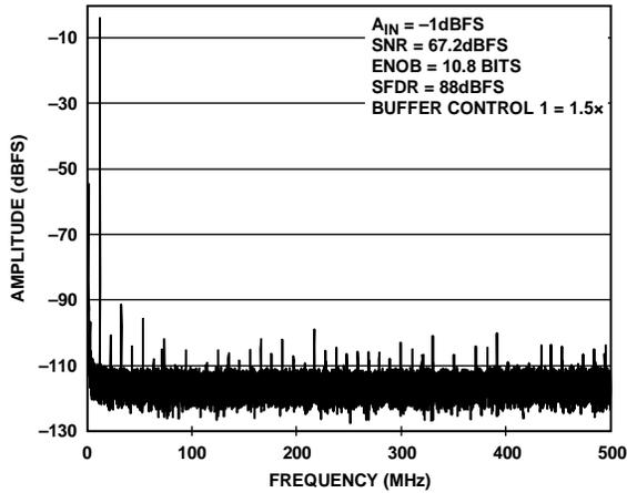
Figure 6. Single-Tone FFT with  $f_{IN} = 10.3$  MHz
