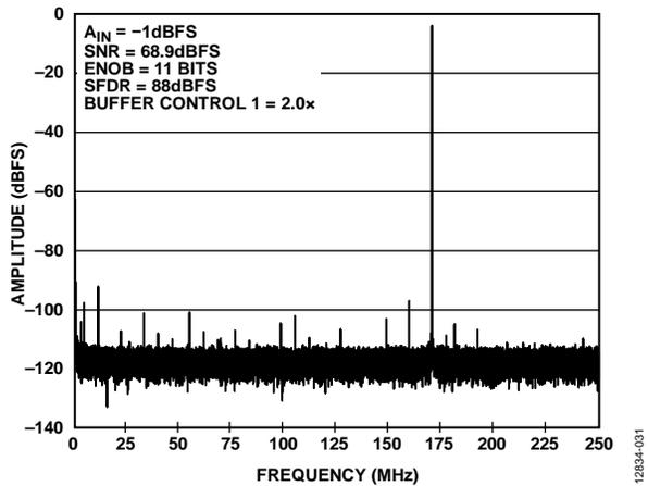
Figure 31. Single-Tone FFT with  $f_{IN} = 170.3$  MHz
