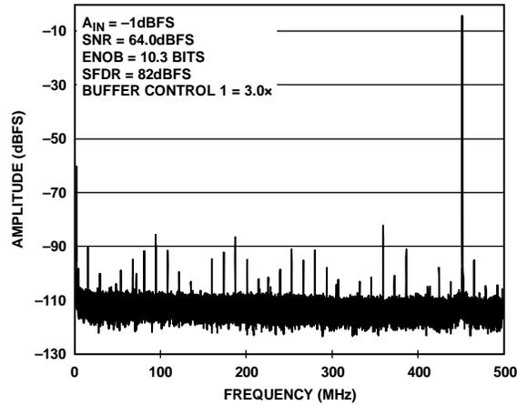
Figure 9. Single-Tone FFT with  $f_{IN} = 450.3$  MHz
