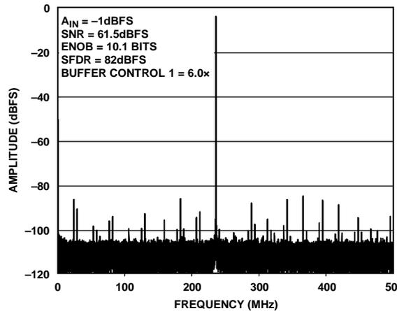
Figure 10. Single-Tone FFT with  $f_{IN} = 765.3$  MHz
