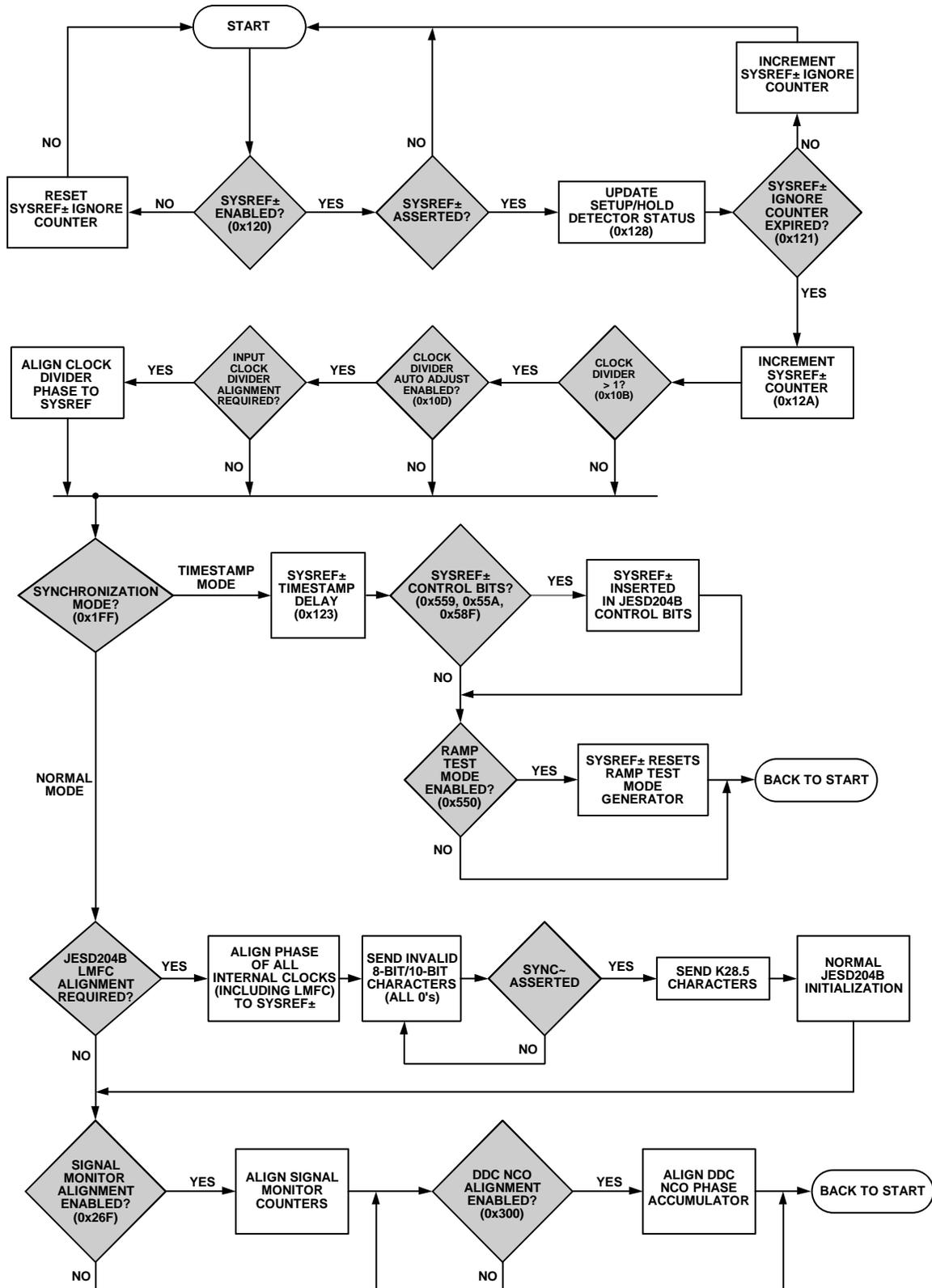
Figure 111. Multichip Synchronization
