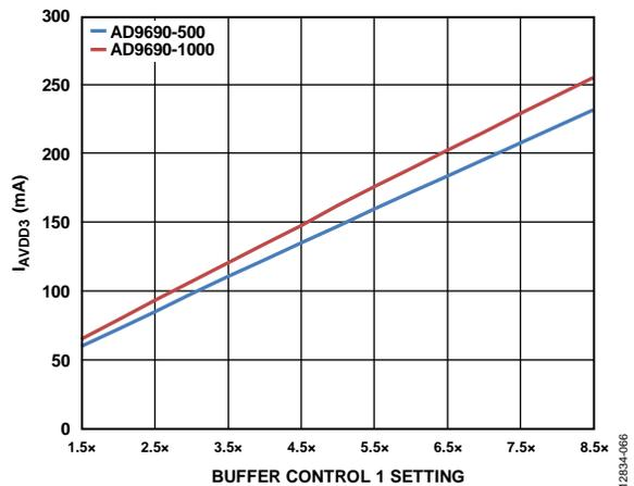
Figure 66. I<sub>AVDD3</sub> vs. Buffer Control 1 Setting in Register 0x018
