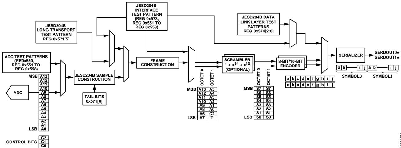
Figure 98. ADC Output Data Path Showing Data Framing
