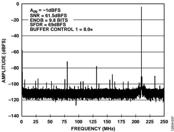
Figure 37. Single-Tone FFT with  $f_{IN} = 1710.3$  MHz
