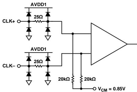
Figure 54. Clock Inputs
