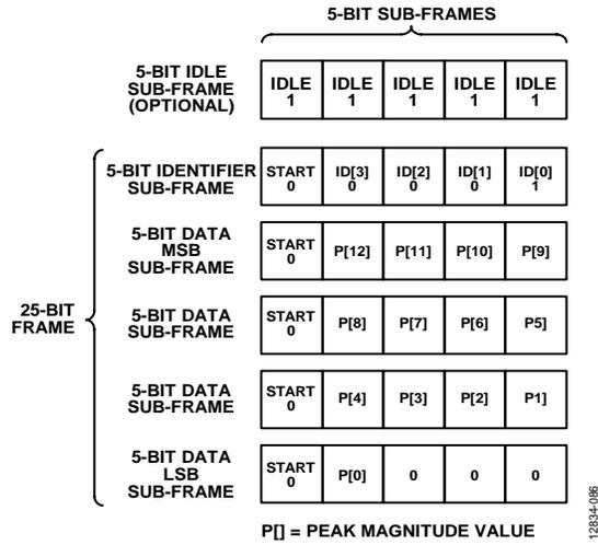
Figure 86. SPORT over JESD204B Signal Monitor Frame Data
