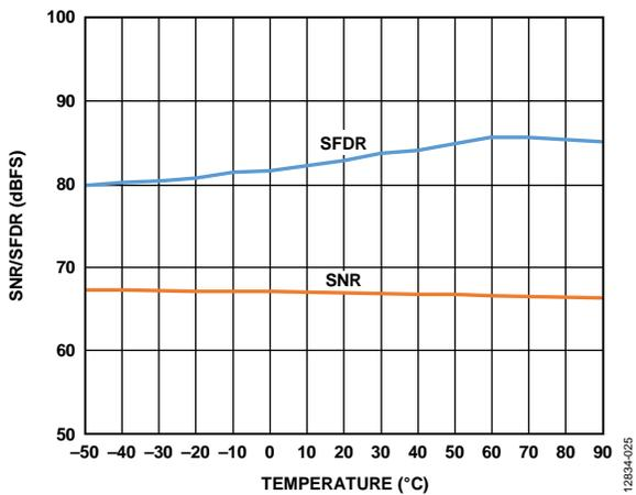
Figure 25. SNR/SFDR vs. Temperature,  $f_{IN} = 170.3$  MHz
