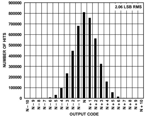
Figure 51. Input-Referred Noise Histogram
