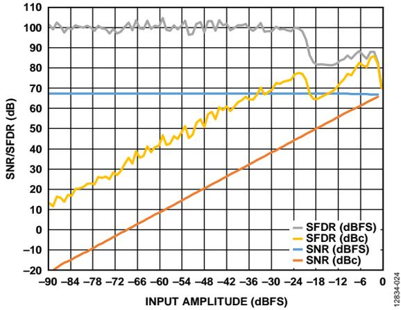
Figure 24. SNR/SFDR vs. Analog Input Level,  $f_{IN} = 170.3$  MHz
