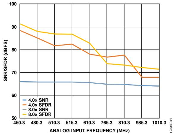
Figure 41. SNR/SFDR vs.  $f_{IN}$ ;  $500$  MHz  $< f_{IN} < 1$  GHz; Buffer Control 1 (0x018) = 4.0x and 8.0x
