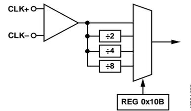
Figure 80. Clock Divider Circuit
