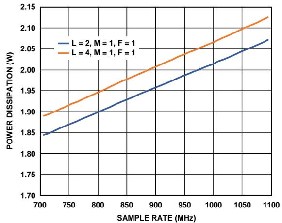
Figure 29. Power Dissipation vs. Sample Rate ( $f_s$ )
