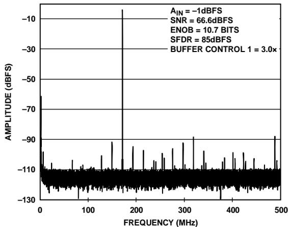
Figure 7. Single-Tone FFT with  $f_{IN} = 170.3$  MHz
