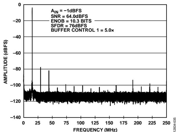
Figure 35. Single-Tone FFT with  $f_{IN} = 985.3$  MHz
