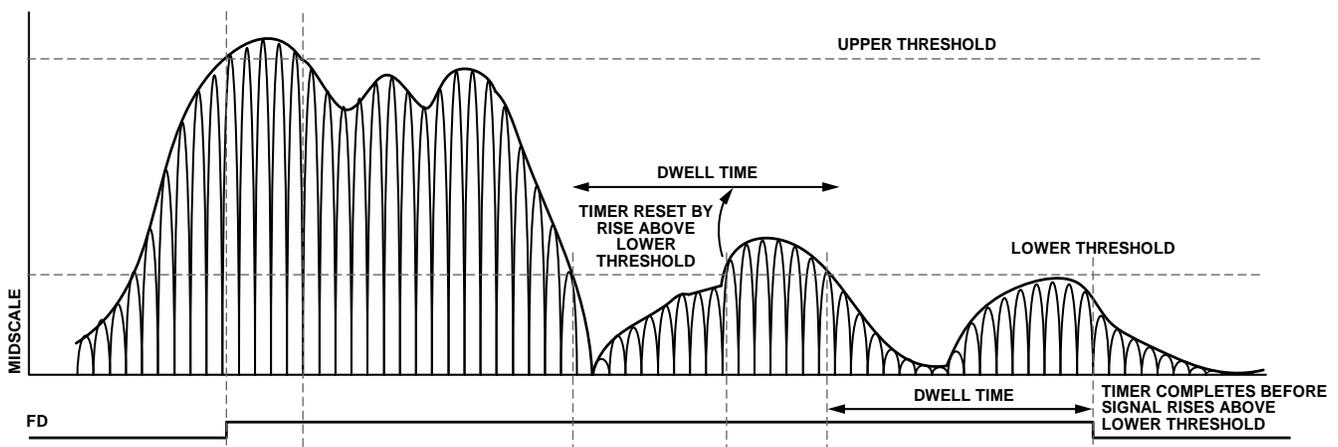
Figure 83. Threshold Settings for FD Signals
