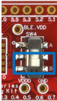
Figure 4-17. SW4 Position for Programming EZ-BLE
