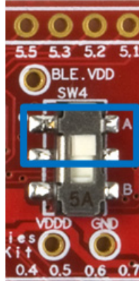
Figure 4-17. SW4 Position for Programming EZ-BLE
