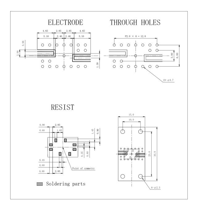
Note: Impedance of signal lines should be 50 ohms including land pattern. This standard condition is applying to the BT resin board (t = 0.4, dielectric constant = 3.6, copper plating on both surfaces).
