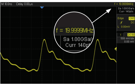
Built-in arbitrary waveform at 20 MHz, 300 MSa/s
