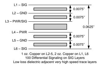
Figure 57. Recommended PCB Layer Stack-Up for a Six-Layer Board
