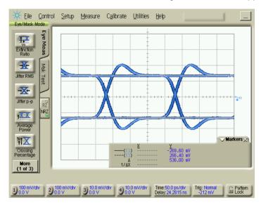
Figure 32. De-emphasis of the Differential Output Signal
