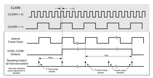
Figure 8. Over-Range Timing Diagram
