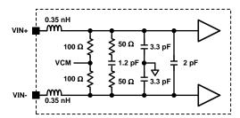
Figure 38. Simplified Analog Input Network Circuit Model
