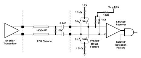
Figure 48. SYSREF Input Receiver and AC Coupled Interface
