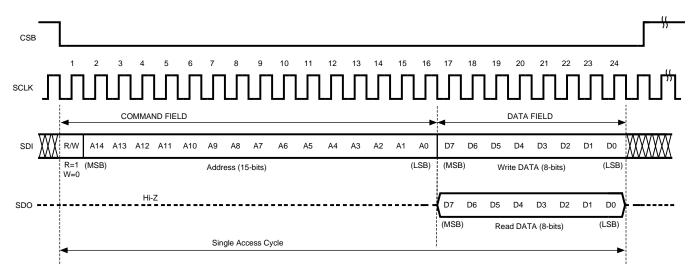
Figure 36. Serial Interface Protocol
