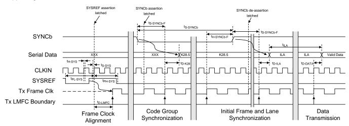
Figure 34. Link-initialization Timing and Flow Diagram
