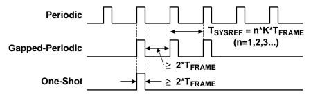
Figure 50. SYSREF Signal Types (Single-Ended Representations)
