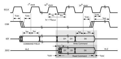
Figure 7. SPI Timing Diagram
