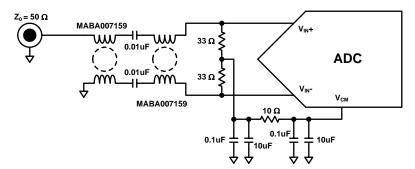
Figure 41. Transformer Input Network
