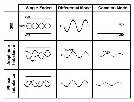
Figure 37. Differential Signal Waveform and Signal Imbalance
