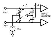
Figure 30. Simplified Input Differential Balance Correction Circuit
