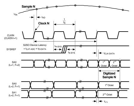
Figure 6. Sample to Data Timing Diagram
