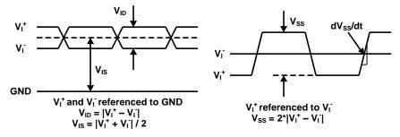
Figure 1. Electrical Level Diagram for Differential Input Signals
