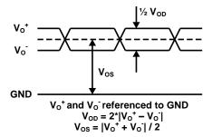
Figure 3. Electrical Level Diagram for Differential Output Signals
