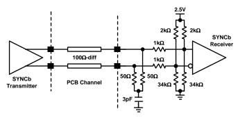
Figure 51. SYNCb Input Receiver and Interface
