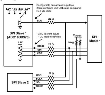
Figure 53. Typical SPI Application
