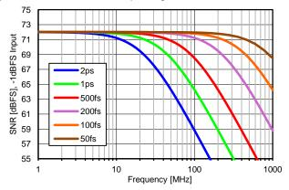
Figure 46. SNR Limit Due to Jitter of Sampling Clock With a Full-Scale Input Signal
