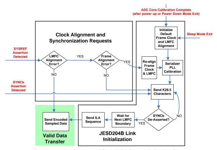
Figure 35. Device Start-Up and JESD204B Link Synchronization Flow Chart
