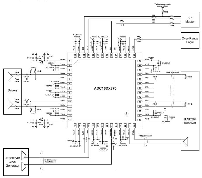
Figure 55. Typical Circuit Implementation
