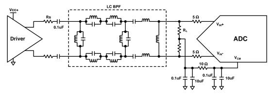
Figure 42. Bandpass Filter Anti-Aliasing Interface
