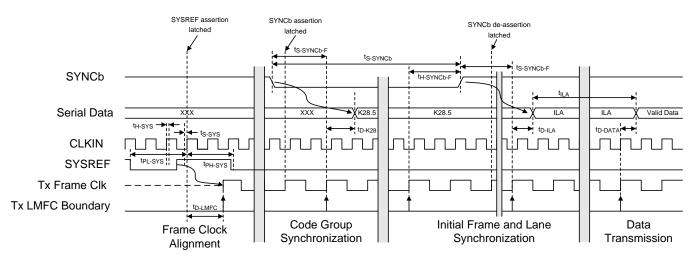
Figure 9. JESD204B Interface Link Initialization Timing Diagram
