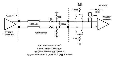
Figure 49. Example DC Coupling to the SYSREF Input
