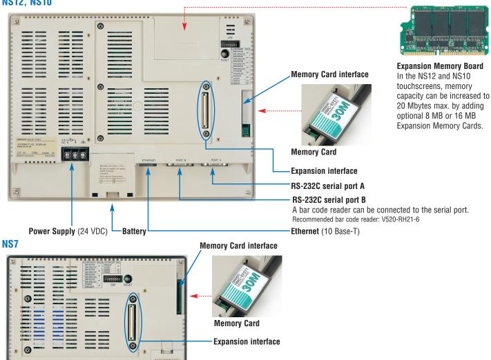
A bar code reader can be connected to the serial port. Recommended bar code reader: V520-RH21-6
